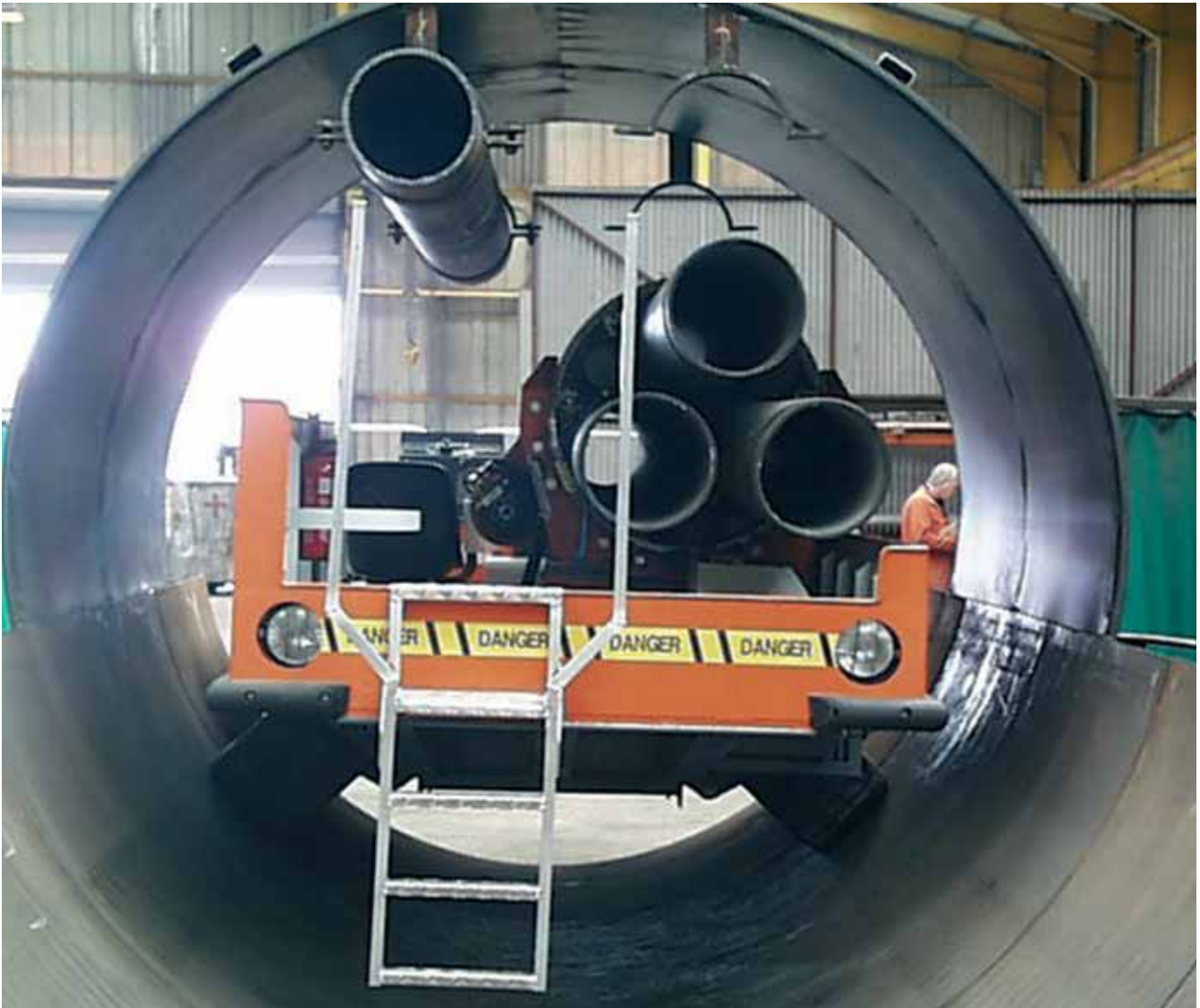
Unique tracked vehicles designed for removing old pipes and fitting new
